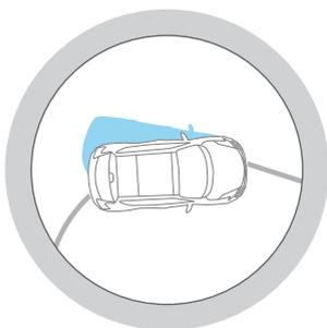
**Vehicle Dynamic Control (VDC).** Also known as stability control, VDC monitors your steering and braking to help you maintain your steered path under certain conditions by reducing engine output and/or applying brake pressure to specific wheels.<sup>6</sup>
