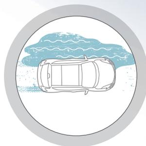
**Traction Control System (TCS).** When TCS senses drive-wheel spin, it responds by reducing throttle or applying brake pressure to help maintain traction.
