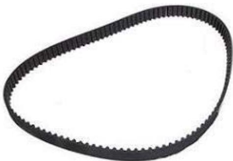
Timing belts resemble an engine accessory serpentine belt in appearance, only they typically have square teeth on the inside surface. They usually are constructed of rubber reinforced with nylon. The timing belt transfers the rotation of the crankshaft to the camshaft. The rotating camshaft activates the valves, which provide air and fuel to the cylinders and expel combustion gases to the exhaust system.
